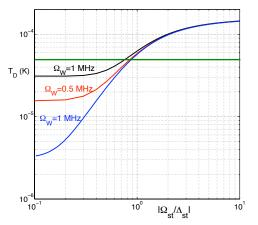
$\Omega_W$  is the Rabi frequency on the 732 nm transition 10 times less scattered photons than for  $S \to P$  Doppler cooling
